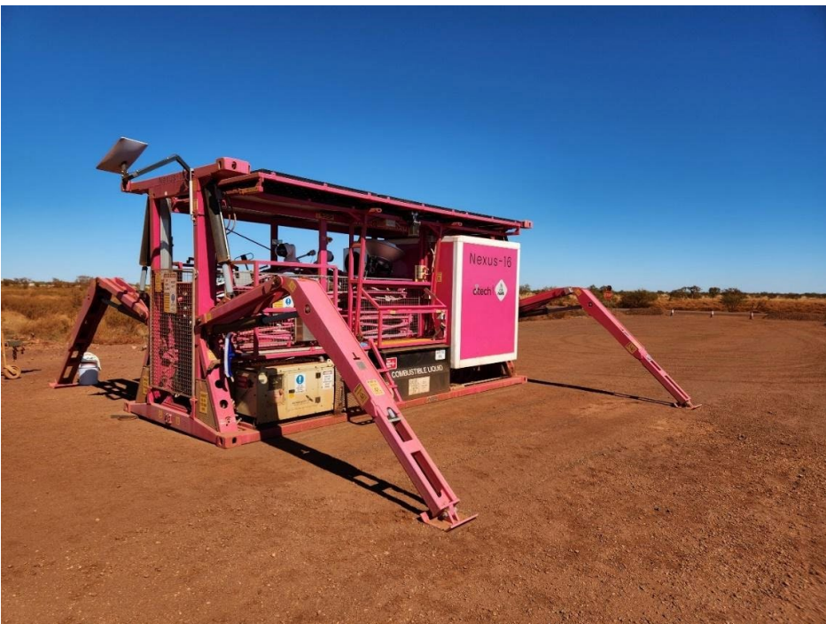
Nexus 16 in "Turtle Mode" ready for the hit — The system secured and retracted, awaiting the cyclone impact.
